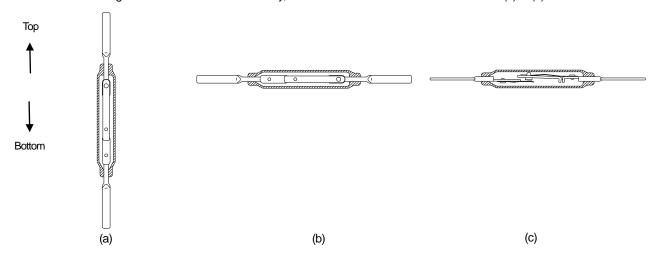
Fig. 2 Installation direction
