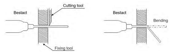
Fig. 3 Pin machining example
